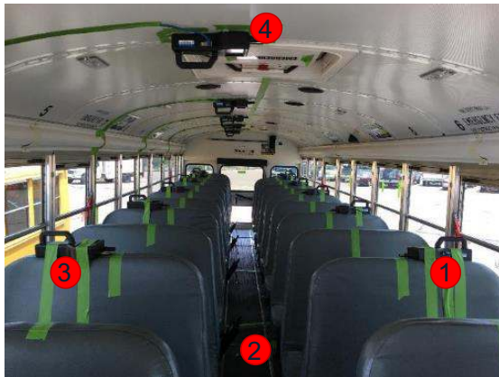
Figure S2: Layout of the school bus sensors: floor, ceiling, and passenger seats. Image on right is showing the mounted location of the anemometer for measuring central airflow.
