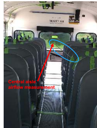
Figure S2: Layout of the school bus sensors: floor, ceiling, and passenger seats. Image on right is showing the mounted location of the anemometer for measuring central airflow.
