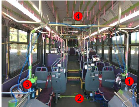
Figure S3: Layout of the transit bus sensors: floor, ceiling, and passenger seats.
