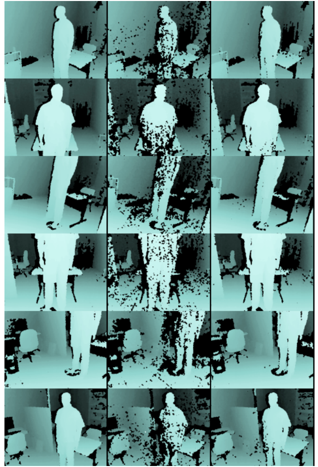
Figure 4: Results for Test Case 2. Rows: Views from six cameras with overlapping views. Left Column: Reference images with no interference, each unit turned on individually. Middle Column: All units operating simultaneously. Right Column: All units operating simultaneously with our interference reduction technique applied.
