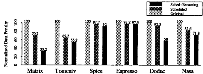
Figure 7: Effect of instruction scheduling on NBC for \delta = 30 ( Pipelined )
