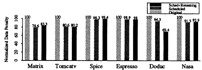
Figure 6: Effect of instruction scheduling on NBC for \delta = 30 ( Non-overlapped )
