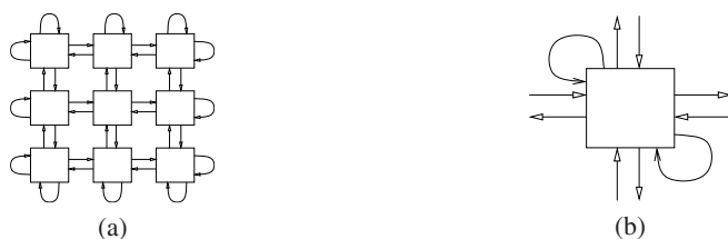
Fig. 2. (a) A closed 3 \times 3 mesh, external output ports are connected to their corresponding input port. (b) A switch with two extra loopback channels.
