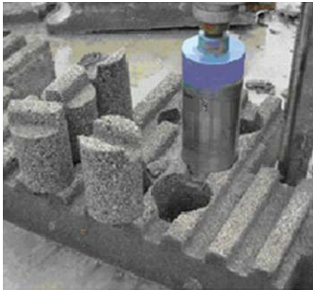
FIGURE 19: Field core from a porous sound-absorbing concrete slab.
