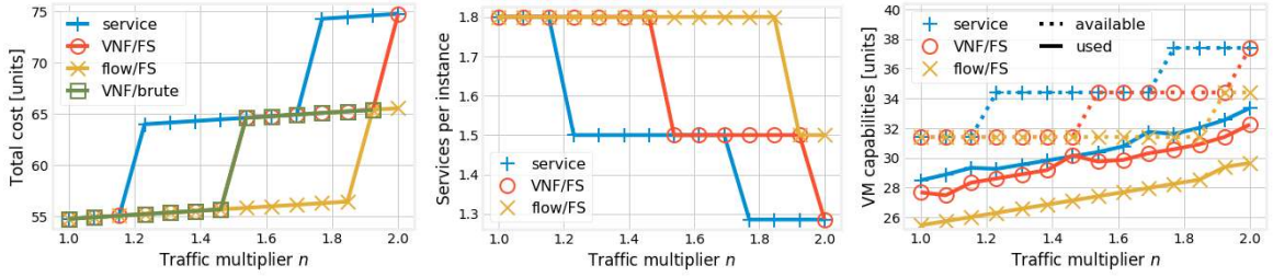
Fig. 9. Synthetic scenario: total cost (left); average number of services sharing a VNF instance (center); used and maximum VM capability (right). Per-VNF and per-flow priorities are assigned via FlexShare; per-service priorities are assigned by giving higher priorities to lower-delay services.
