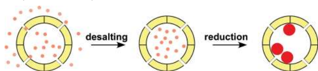
SCHEME 1. Preparation of Apoferritin-Encapsulated Platinum Nanoparticles (Pt-apo)
