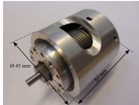
Figure 1. A photograph of the BIC-PEA. It weighs 202 g and fits in a cylinder with a length of 51 mm and a diameter of 45 mm.
