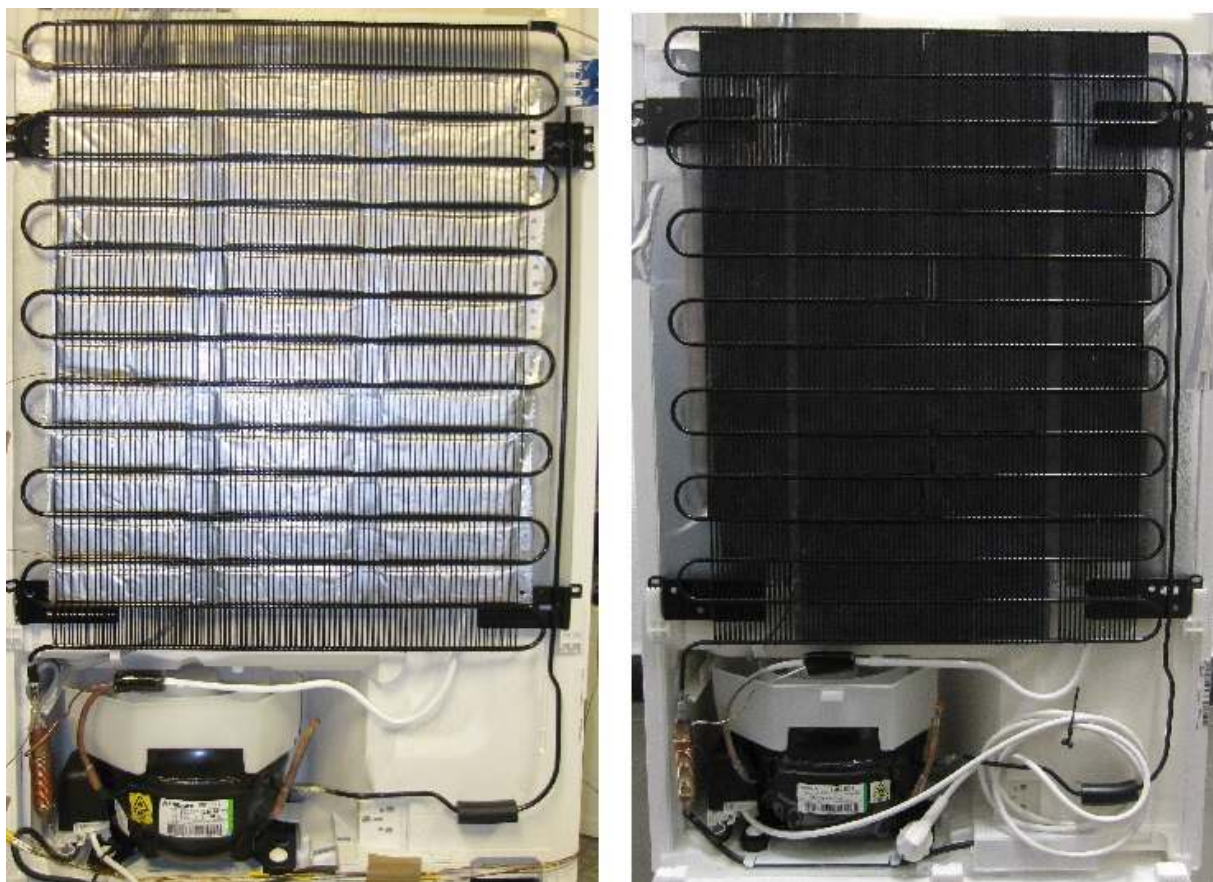
Fig. 1 – Wire-and-tube condenser, equipped with taped bags out of aluminum-composite film (left) or copolymer compound (right)
