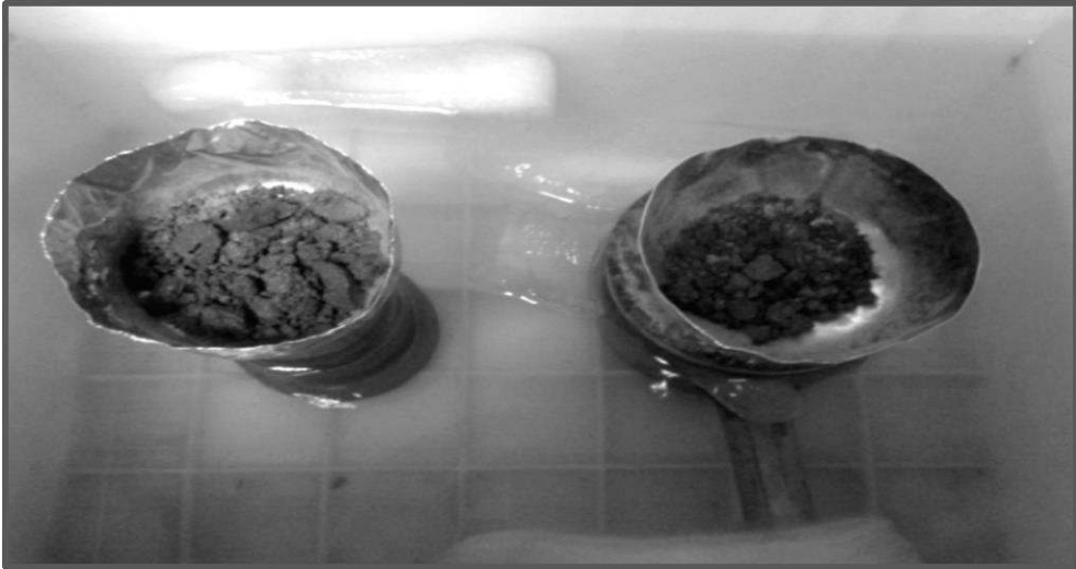
Figure 3: Produced laboratory clinker samples
