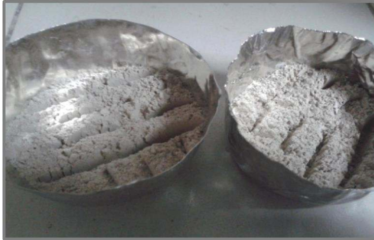
Figure 2: Raw meal preparation for lab clinker production
