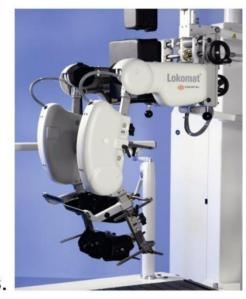
Figure 1 (A). The Lokomat, an automated gait orthosis on a treadmill with a body weight-support system; (B). Lokomat leg orthosis.
