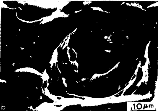
Figure 2 Scanning electron micrographs of beryllium irradiated at 600^\circ\text{C} with 100 keV ^4\text{He}^+ ions. (a) beryllium vacuum-cast from powder irradiated to a dose of 0.5 \text{ C cm}^{-2} , (b) an enlarged view of one of the exfoliated areas in (a), (c) sintered beryllium powder irradiated to a dose of 1.0 \text{ C cm}^{-2} .
