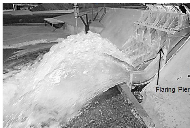
Figure 11. Test performed with Flaring Piers (Alternative 9) for flow with a 100-year recurrence.
