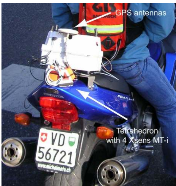
Fig. 14: SRIMU installed on a motorcycle.
