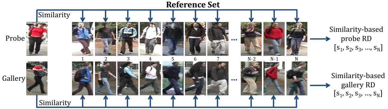
Figure 4. The reference descriptor (RD) for a probe/gallery subject is generated by computing the similarity between the probe/gallery data and each of the subjects in the reference set. N is the number of subjects in the reference set and s_i is the similarity between the probe/gallery and the i^{th} subject in the reference set.
