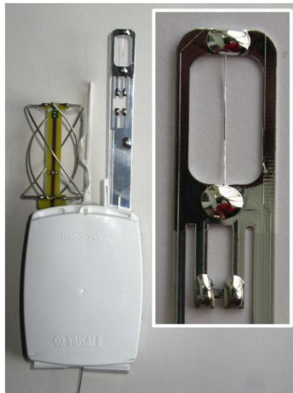
Figure 1. Photograph of the RS92 radiosonde showing the GPS antenna on the left and the sensor boom on the right. The inset shows the magnified tip of the sensor boom with the wire-shaped temperature sensor and one of the humidity sensors.
