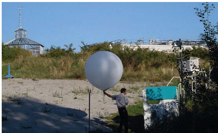
FIG. 2. The Deutscher Wetterdienst’s Meteorologisches Observatorium Lindenberg, designated as GRUAN Lead Center and the first GRUAN network station, has all the GRUAN observational capabilities depicted in Fig. 1. Here Michael Schröter prepares to launch a radiosonde and verifies that the ground station is receiving data from the sonde. A Stevenson shelter (behind bushes at lower right) houses reference surface instruments for comparison. On the roof of the radiation building (in background on right) are Baseline Surface Radiation Network instruments (pyranometer, pyrhelimeter, pyrgometer, and all-sky camera) and a microwave radiometer (far right). A GSNN antenna is to the left of the radiation building. The historic winch house (in background on left) was used in the nineteenth and twentieth centuries for meteorological profile observations with tethered aerological kites; the observatory holds the world record for achieving a kite altitude of 9,750 m on 1 Aug 1919.
