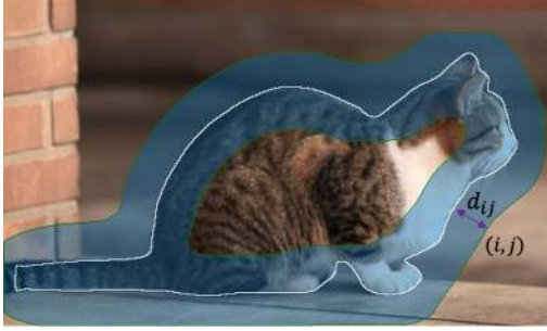
Figure 4: An illustration of object boundary region. d_{ij} is defined as the Euclidean distance from pixel p_{ij} to its nearest pixel on the mask contour (the white line).
