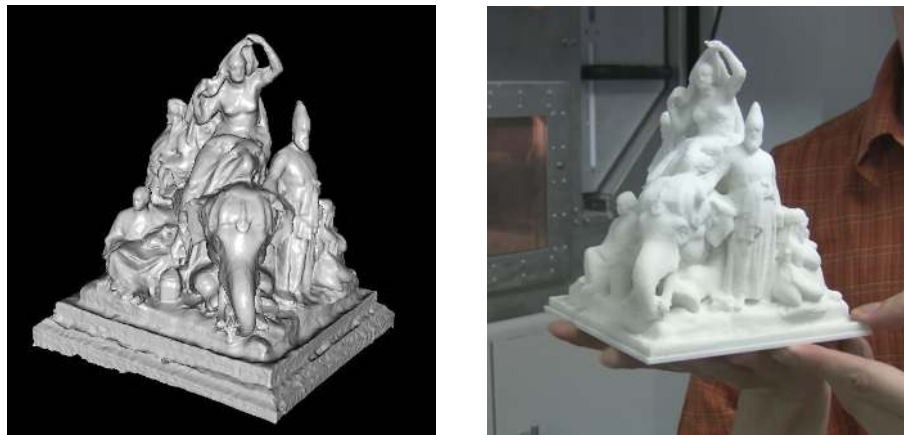
Fig. 7. Results on the Asia dataset. Left: initial model produced with depth map fusion [1]. Right: replica produced with rapid prototyping from the final model refined by our method.
