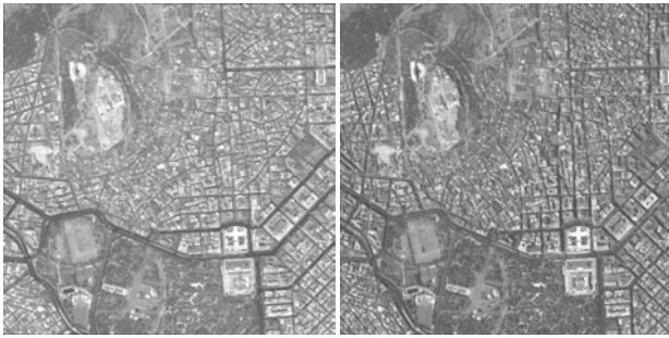
Figure 7. Section 1500 m × 1500 m from the Athens Stere scene, left and right stereo image showing the Acropolis (left top)
