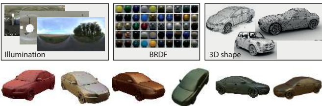
Fig. 7. Our dataset for the reflectance map estimation consists of synthetic images with random view, 3D shape, material, illumination, and exposure.
