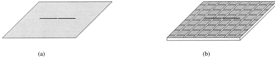
Fig. 2. Dipole antenna over (a) the PEC or PMC ground plane or (b) the EBG ground plane.
