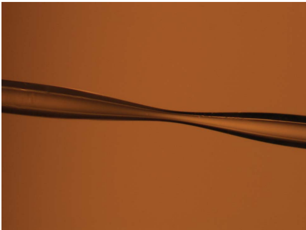
Fig. 2. (Color online) One 3 dB taper made by a fusion splicer.
