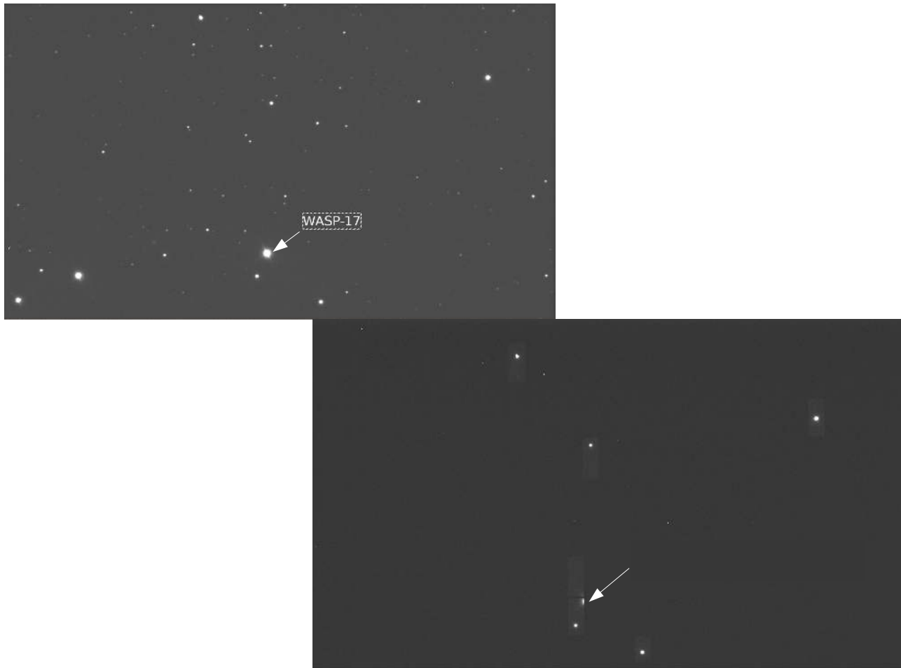
Figure 3. An unfortunate case where no useful data could be obtained. In this case, the instrument is not to blame, as it seems that the observer forgot to do pre-imaging, and possibly underestimated the proper motion of the target (indicated by the arrow), and so did not centre precisely enough the (wide) slits. The upper image is the acquisition image, while the lower one is the through-slit image.
