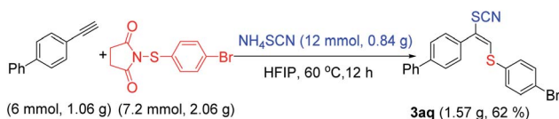
Scheme 2 Gram-scale preparation of 3aq .
