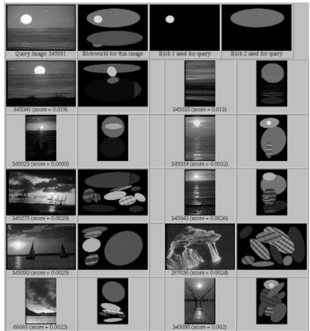
Figure 6. Query for sunset images. 62% of the top 50 images are sunsets; about 5% of the images in the database are sunsets.
