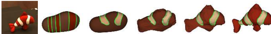
Fig. 1. (COLOR) A plush model of “nemo.” The object exhibits piecewise constant appearance. From a set of calibrated views, our algorithm can estimate the shape and the piecewise constant radiance.
