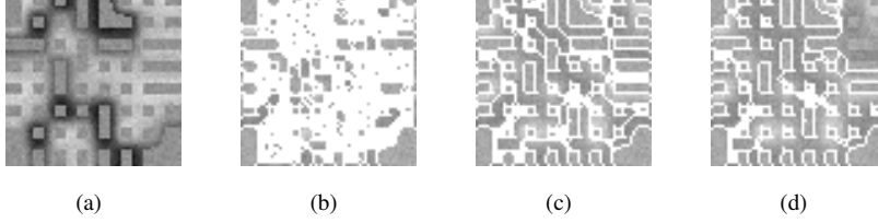
Fig. 5. Segmentation results. (a) Synthetic data of band 100. (b) Segmentation of band 100 with T = 10 . (c) Segmentation of band 100 with T = 50 . (d) Segmentation of band 100 with T = 200 .
