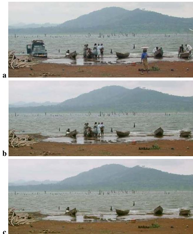
Fig. 24. Removing several objects from a photograph. (a) Original image, a photograph from Ghana. Courtesy of P. Anandan. (b,c) The crowd of people and other objects are gradually removed by our algorithm. The source regions have been selected as dilated bands around the target regions. Background texture and structure have seamlessly replaced the original characters.
