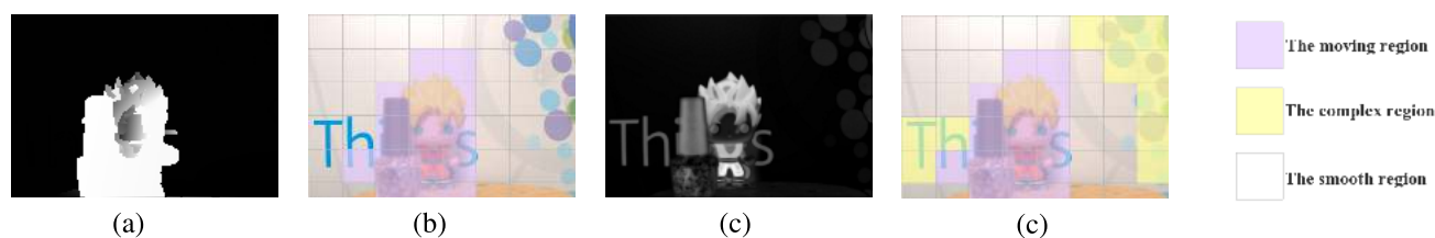
FIGURE 8. Results of the proposed region division method (The centre view's first frame of Bottle sequence, and the largest size of coding units is 64 \times 64 ): (a) Moving region distribution map, (b) Moving region division result, (c) Texture distribution map, (d) Non-ROI sub-division result.
