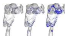
Figure 5. Oral airway deposition patterns for 2.5, 10, and 30- \mu\text{m} particles with respective deposition efficiencies of 3.9%, 9.5%, and 75.0% (left, middle, right)
