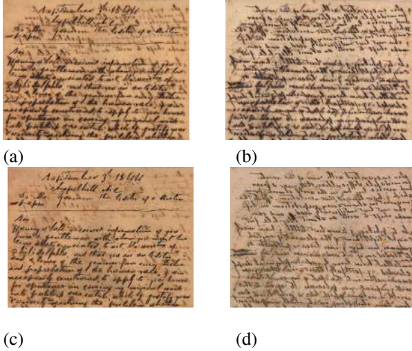
Figure 1. Restoration of a real recto-verso RGB pair: (a) recto; (b) flipped verso; (c) restored recto; (d) flipped restored verso.
