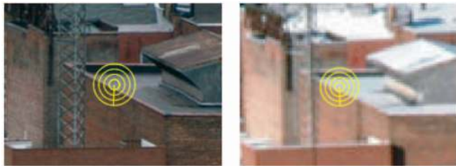
Fig. 3. Initial keypoint match and side-by-side alignment for a summer-winter pair. The image region on the right has been scaled by a factor of 2.25 and there are substantial illumination, blurring, and physical changes (snow) between the regions.
