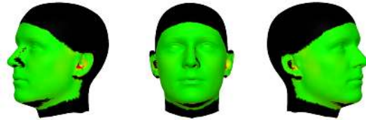
Figure 6. Average distance of the vertices from the original surface, ranging from 0.0 mm (green) to \geq 1.0 mm (red). The black areas correspond to vertices missing in at least one example. Most of the vertices are close to the surface.
