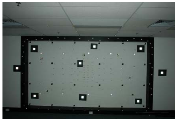
Figure 3. The calibration wall comprised of retro-reflective targets.
