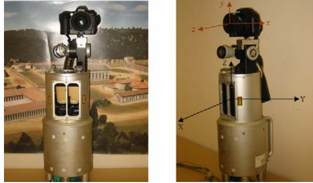
Figure 1. The Nikon D100 camera rigidly attached to the Riegl TLS.
