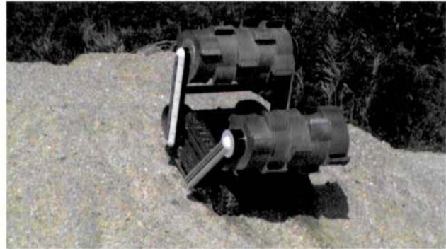
Figure 6 – Driving up a 20 degree slope of loose crawler-way fines.
