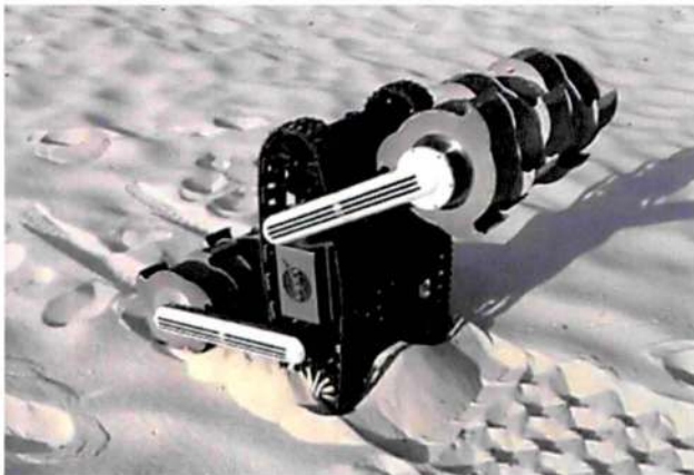
Figure 5 – RASSOR in the “Z” position demonstrating its ability to dump sand.
