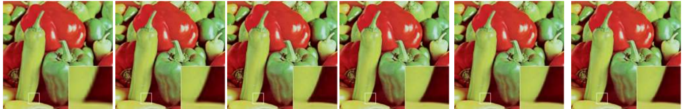
Bicubic / 32.39 dB ANR / 33.82 dB SRCNN / 34.35 dB JOR / 34.65 dB A+ (1024 r.) / 34.73 dB RB (32 br.) / 34.66 dB Fig. 4. ‘Pepper’ image from Set14 with upscaling \times 3 . Best zoomed on screen.
