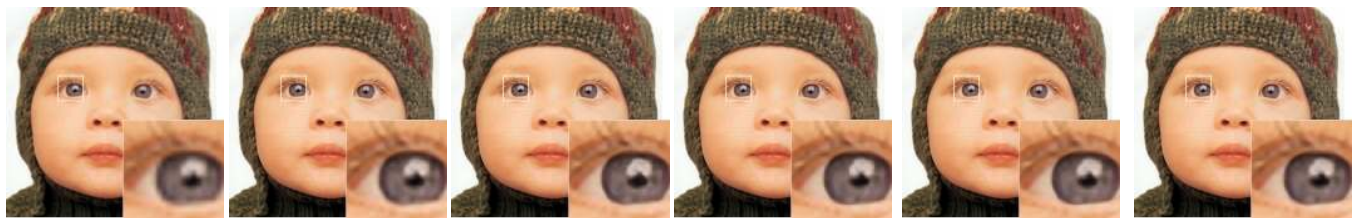
Bicubic / 33.91 dB ANR / 35.13 dB SRCNN / 35.01 dB JOR / 35.23 dB A+ (1024 r.) / 35.21 dB RB (32 br.) / 35.30 dB Fig. 3. ‘Baby’ image from Set5 with upscaling \times 3 . Best zoomed on screen.
