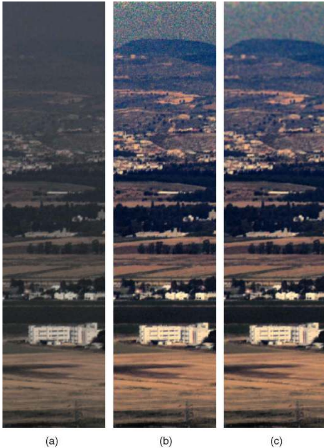
Fig. 4. (a) Raw frame. (b) Simple inversion. (c) Adaptive regularization attenuates noise at the background, while sparing consequent blur from foreground objects.
