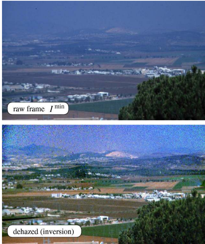
Fig. 1. Top: An image of a hazy scene, corresponding to the best state of mounted polarizer. Bottom: Dehazed image, using the basic algorithms of [17]. While contrast is significantly improved, noise is amplified in pixels corresponding to long distances.
