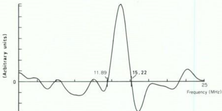
Figure 3. Fourier cosine transform of shortened data record ( \tau=0.04 \mu\text{s} ).
