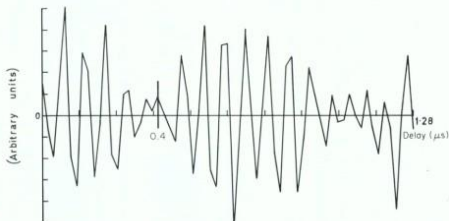
Figure 1. Autocorrelation function near a shock wave.
