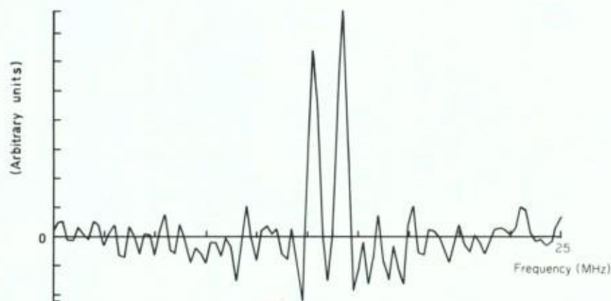
Figure 2. Fourier cosine transform of data of figure 1; peaks at 12.80 and 14.23 MHz.
