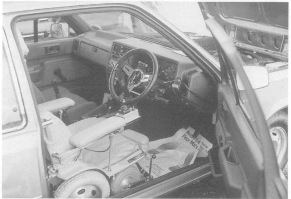
Fig 2 A variety of both simple and complex adaptations are now possible to enable an individual with severe physical disabilities to safely control a motor vehicle
