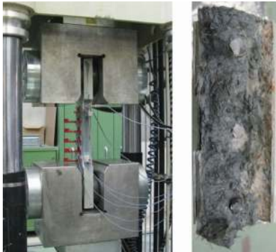
Figure 7. Tensile fatigue test set-up on plain and R-UHPFRC; fracture surface of R-UHPFRC (dimensions: 40 \times 110 \text{ mm}^2 ).
