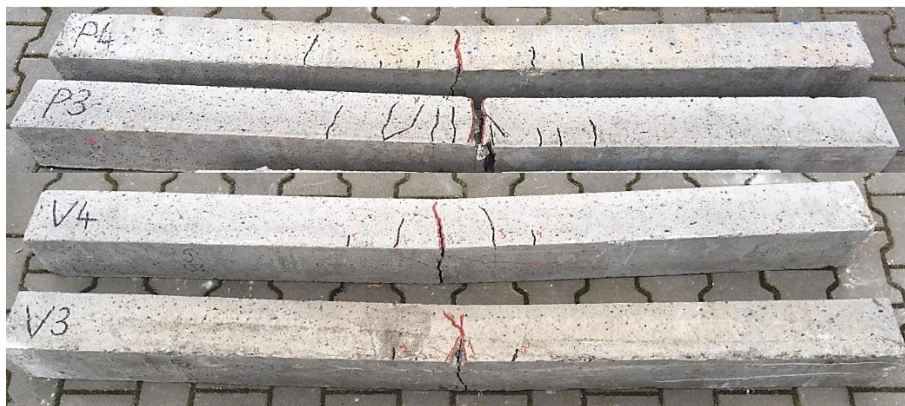
Fig. 9: Crack mesh on beams after collapse P3, P4, V3 and V4.
