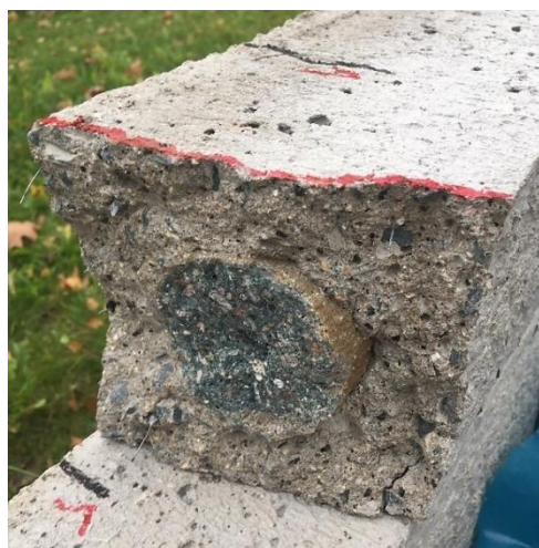
Fig. 4: Detail of the post-filled beam with alkali-activated material.
