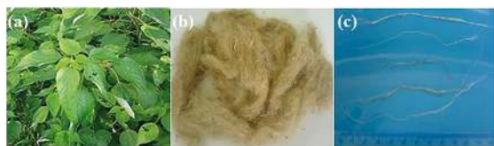
Figure 1. The typical ramie plant (a), bunch of ramie fibers (b) and separated ramie fibers (c).
