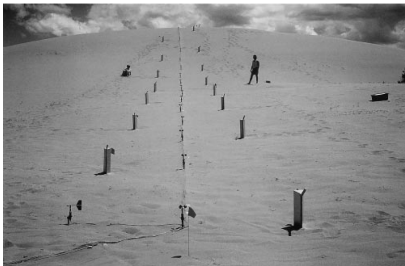
Fig. 3. View of typical array of anemometers and sand traps on a study dune (D13, north slope).
