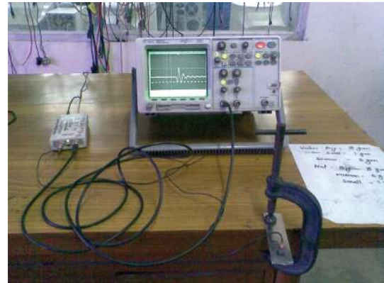
FIGURE 4: Experimental setup for the determination of damping factor.
