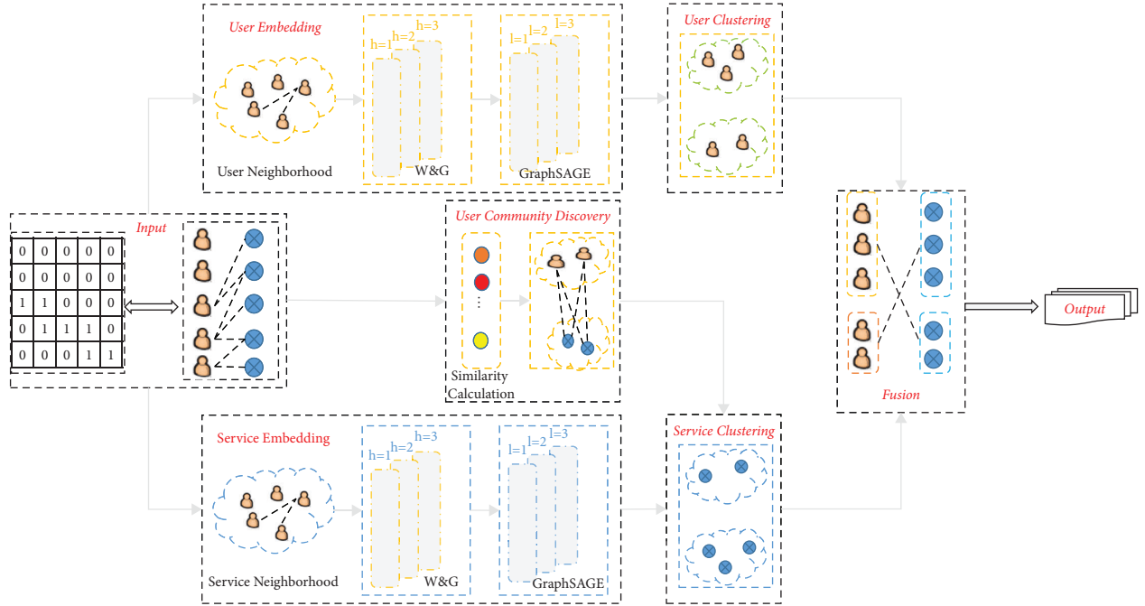
FIGURE 2: The framework of web service quality prediction. The input can be QoS matrix or corresponding bipartite graph. The output is the prediction of missing QoS values.
