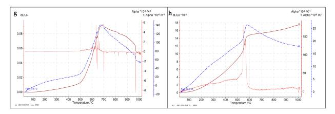
**Figure 7.** Linear thermal expansion (LTE) patterns showing the behavior of different granitic rocks under increasing temperatures: (a) gandonna; (b) pink granite; (c) buff granite I; (d) buff granite II; (e) fantazia; (f) red granite; (g) rosa granite; (h) qusseir brown.
