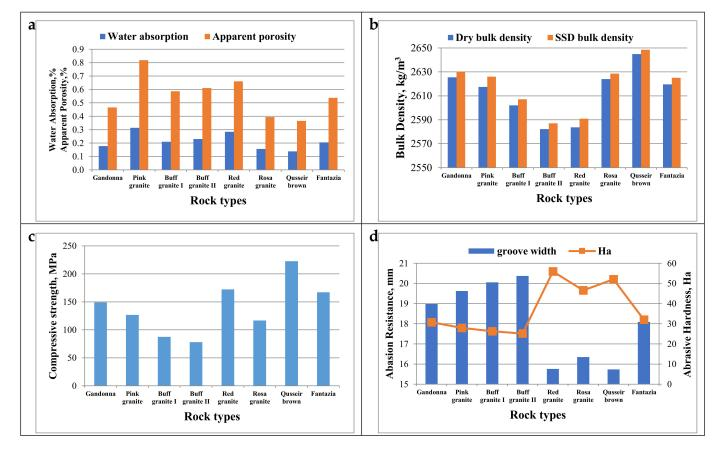
Figure 11. Physico-mechanical properties of different granitic rock types. (a) water absorption and porosity; (b) dry and saturated surface dry (SSD) bulk density; (c) compressive strength; (d) abrasion resistance.
