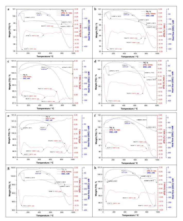
**Figure 6.** Thermogravimetric analysis of different granitic rocks using TG/DTG/DSC: (**a**) gandonna; (**b**) pink granite; (**c**) buff graniteI; (**d**) buff graniteII; (**e**) fantazia; (**f**) red granite (**g**) rosa granite; (**h**) qusseir brown. A circle shape represents the phase transition of  $\alpha$ - $\beta$  quartz at 573 °C.
