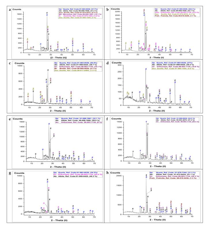
**Figure 5.** X-ray diffraction (XRD) patterns showing the main mineralogical composition of different granitic rocks: (a) Gandonna; (b) pink granite; (c) buff graniteI; (d) buff graniteII; (e) Fantazia; (f) red granite; (g) Rosa granite; (h) Qusseir brown.
