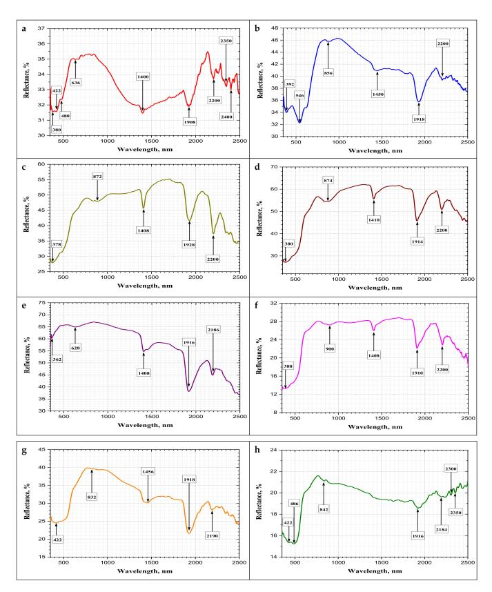
**Figure 9.** Spectral reflectance patterns in VIS-NIR and SWIR regions (350–2500 nm) of different granitic rocks: (**a**) gandonna; (**b**) pink granite; (**c**) buff granite I; (**d**) buff granite II; (**e**) fantazia; (**f**) red granite; (**g**) rosa granite; (**h**) qusseir brown.
