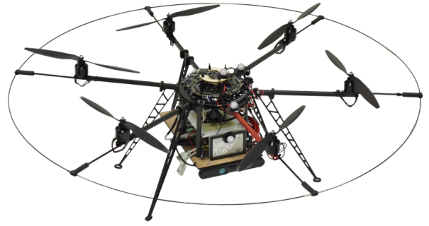
Fig. 1. The Mikrokopter hexacopter that is used to carry out the experiments. The only sensors utilized are an altimeter (not visible), IMU, and front-facing RGB-D camera.
