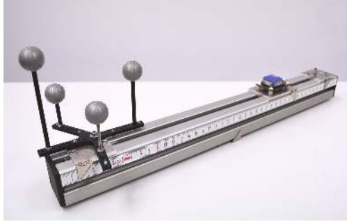
Fig. 3. 45 cm long rigid beam mounted with OT and IMU
