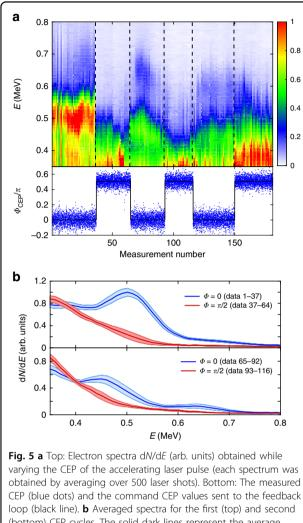
(bottom) CEP cycles. The solid dark lines represent the average spectra, whereas the light blue and red areas indicate the standard deviation due to spectral fluctuations
